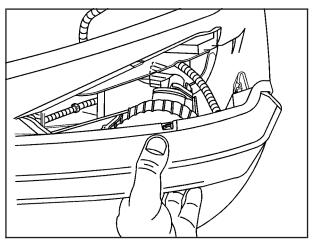
3. Pull the turn signal housing out from the vehicle.
